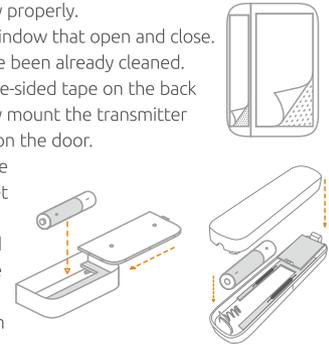
**Note!** The door sensor is set in Normal Zone1 as default. It will cause an immediate alarm if the magnet departs from the transmitter more than 2cm in arming state.
