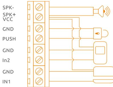
1. Connect one wire to IN1 or IN2 block while another to GND block. If no power supply is needed for wired sensor, don't connect to VCC block.
