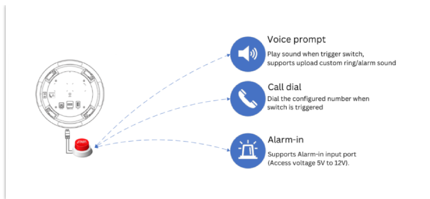
2-pin Multi-Purpose Input Applications for GSC3506
